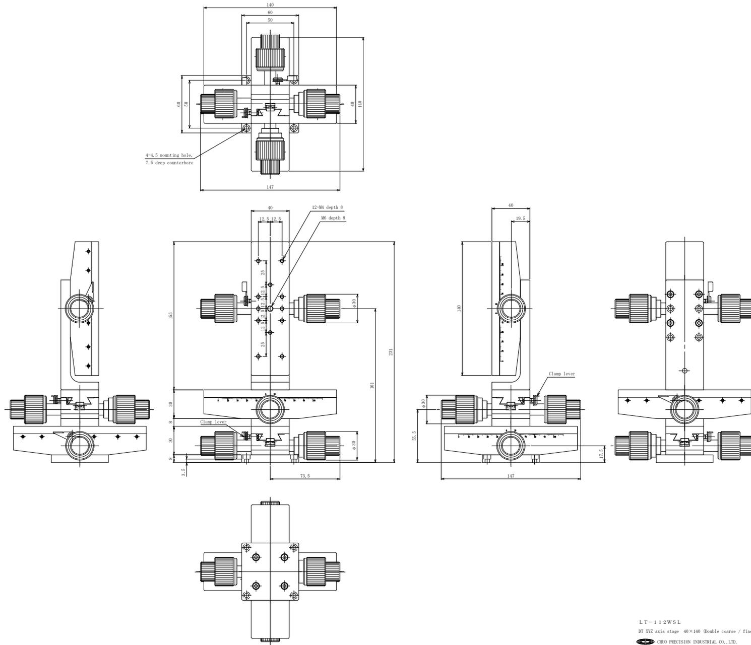
\*Mounting screw : Hexagon socket head cap screw M4, 4 screws
