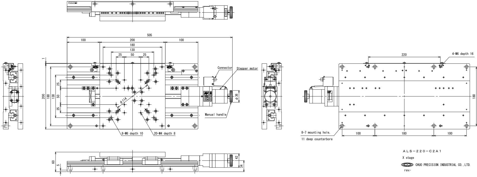
\*Mounting screw : Hexagon socket head cap screw M6, 8 screws
