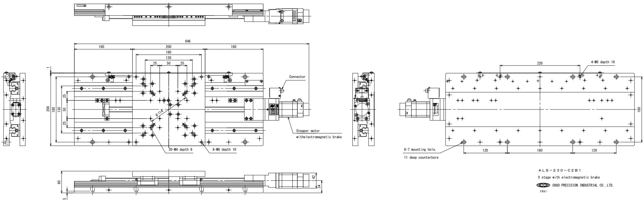
\*Mounting screw : Hexagon socket head cap screw M6, 12 screws
